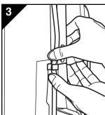
Attach cord assembly to cord clip by pressing cord above and below clip ensuring the cord is fully rested in clip.
